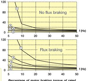
Percentage of motor braking torque of rated torque as a function of output frequency
