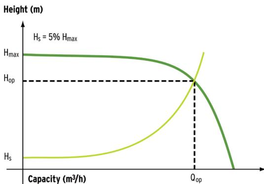
Pump systems are typically designed to ensure a guaranteed target maximum operational flow ( $Q_{op}$ ). An ideal pump will be chosen to operate at its BEP at the operational flow.
