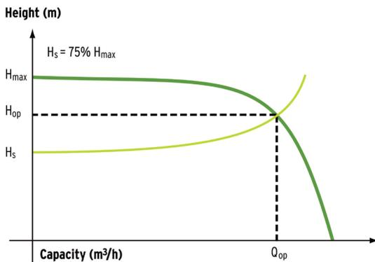
**Figure 3: Hydraulic system with low static head**
