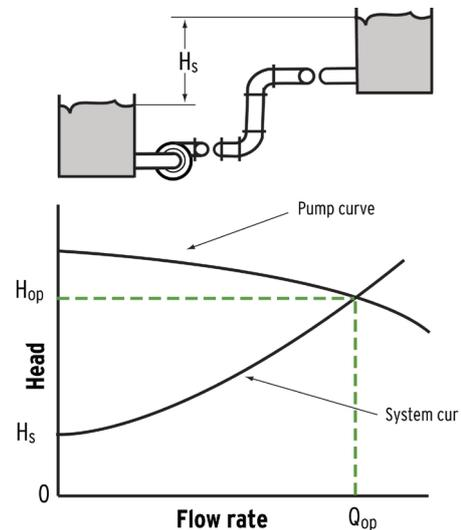
The design and characteristics of each type of pumping system can vary widely and so can the way the energy usage and losses are distributed within the system. For example, in a static head dominant system (**Figure 2**), most of the energy is used elevating the liquid to the desired head or height.
