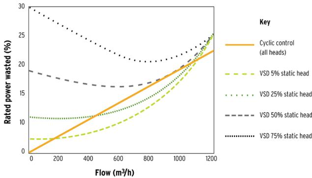
The results of this investigation are compelling: **Cyclic control is the most efficient method of control for applications with medium to high static head.** Even at the relatively low static head of 25%, there is little overall difference in efficiency between real-time flow control and cyclic control. Real-time flow control becomes increasingly inefficient for higher static heads. These results agree with the conclusion presented by ABB [2].
